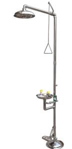
Eye wash shower Foot operated, Body shower Hand operated Suitable to be attached to the ground with its own footplate Shower bowl stainless steel 300 mm All pipes are made of stainless steel
